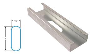
First punchout is centered 12" from beginning of member; subsequent punchouts are 24" on center (o.c.). Center of last punchout is no less than 12" from end of member.
