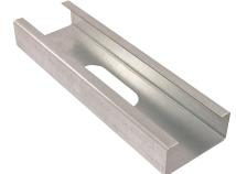
First punchout is centered 12" from beginning of member; subsequent punchouts are 24" on center (o.c.). Center of last punchout is no less than 12" from end of member.
