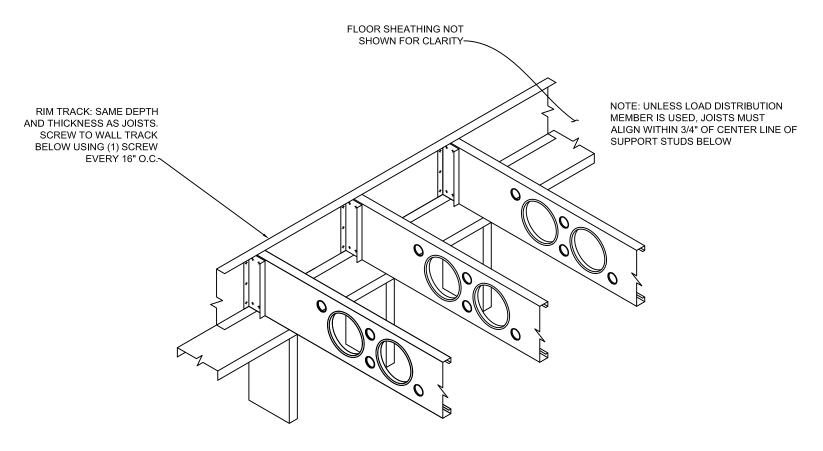
WEB STIFFENERS: USE MIN 54 MIL X 4" DEEP X 1 1/4 FLANGE SEGMENT OF STUD OR TRACK. STIFFENER MAY BE UP TO 1/2" LESS THAN JOIST HEIGHT
