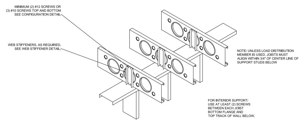
WEB STIFFENERS: USE MIN 54 MIL X 4" DEEP X 1 1/4 FLANGE SEGMENT OF STUD OR TRACK, STIFFENER MAY BE UP TO 1/2" LESS THAN JOIST HEIGHT
